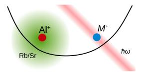
FIG. 1. Schematic representation of the considered experimental arrangement with an  $Al^+$  ion co-trapped in a Paul trap with a laser-cooled alkaline-earth-metal ion  $M^+$ . An  $Al^+$  ion is overlapped with a small cloud of ulracold Rb or Sr atoms, whereas an alkaline-earth-metal ion is optically addressed to control and read a quantum state of both ions.
