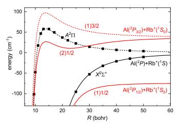
FIG. 6. The long-range part of the interaction potentials for the  $(Al + Rb)^+$  ion-atom system. Points are the result of the supermolecular calculations and lines are the multipole expansion  $-C_3/R^3 - C_4/R^4 - C_6/R^6$  with coefficients obtained within the perturbation theory. Black and red (gray) lines present nonrelativistic and relativistic potential energy curves, respectively.
